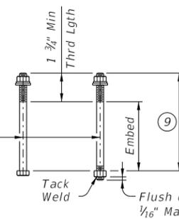
**CAST-IN-PLACE & FORMED HOLE ANCHOR BOLT OPTIONS (10)**
