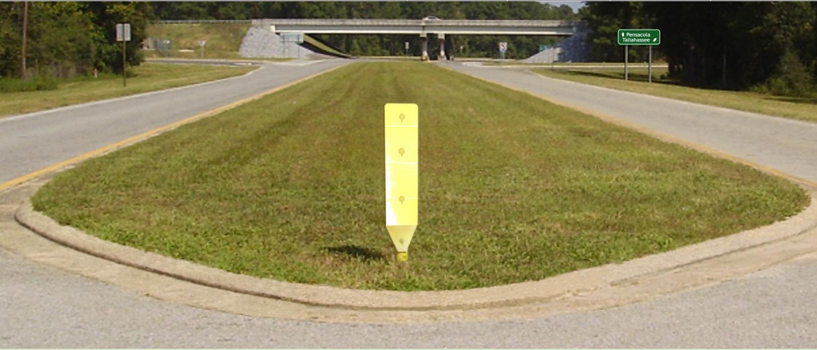
The Dura-Post® VP, High Performance Vertical Panel, is designed to meet the most demanding requirements for high visibility, reboundable sign systems. The Dura-Post VP has been successfully tested to withstand 10 bumper hit and wheel over impacts at 55mph. The Dura-Post VP is accepted by the Florida Department of Transportation as a High Visibility Median Separator delineation device. (Pictured Above.)
