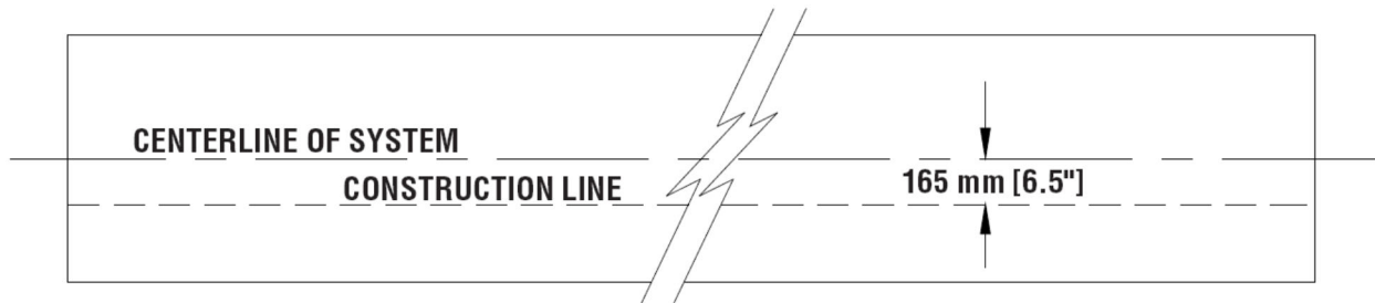
Figure 16 (Top view of concrete pad) Locating Construction Line
