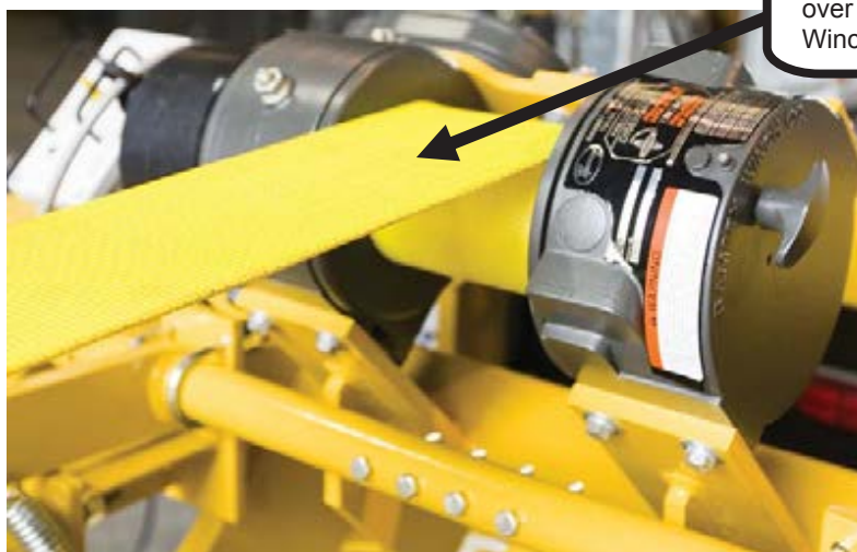
Figure 24.3 Always Locate Strap to Wrap Over Top of Winch Drum
