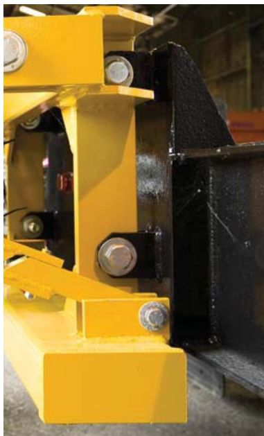
Figure 31.0 MPS 350 Bumper Assembly Bolts Mounting MPS 350 to Truck Frame
