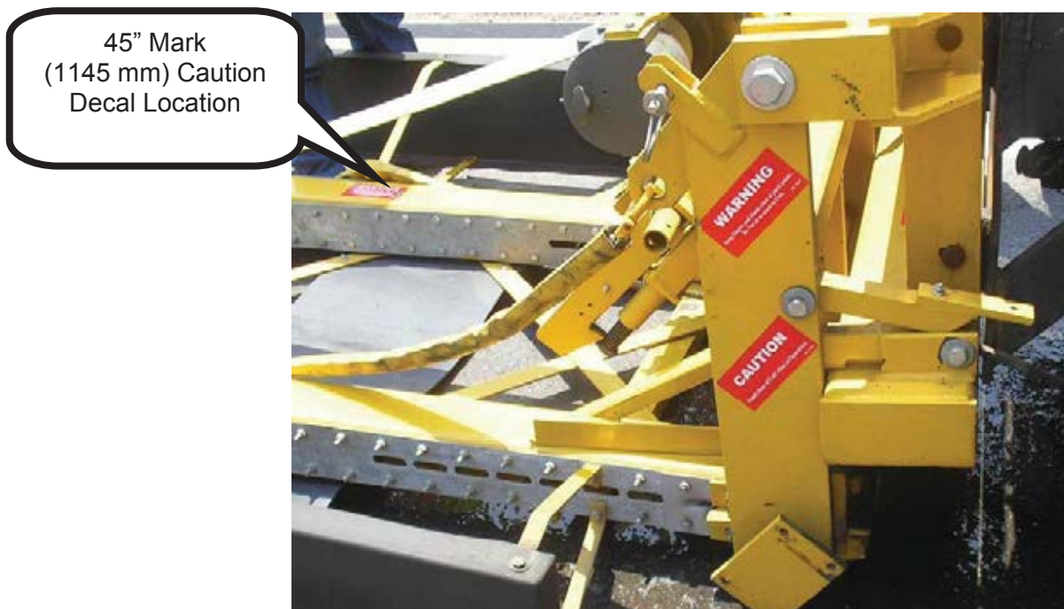
Figure 39.0 Low Speed Impact Ripping Less than 45" (1145mm) of Rip Plates
