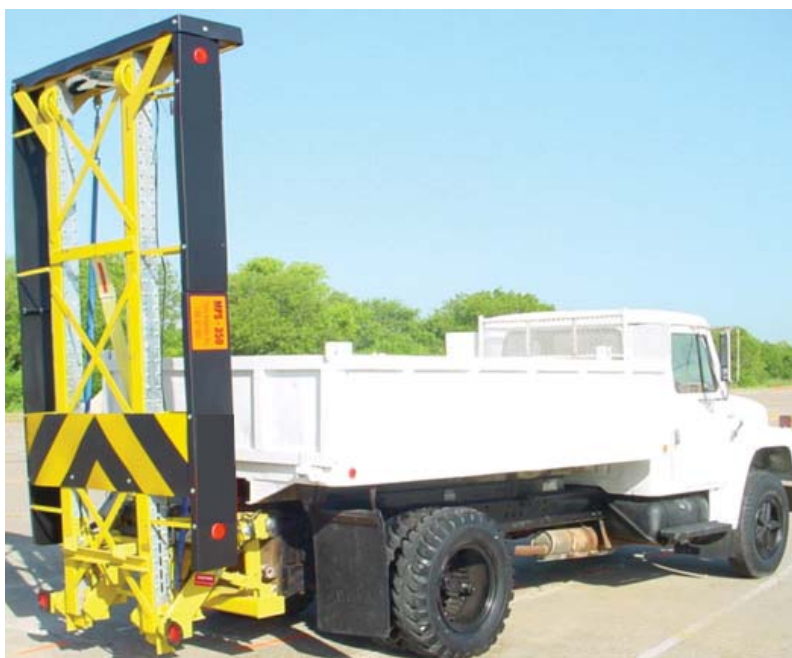
Figure 18.0 MPS 350 in Up (Traveling) Position
