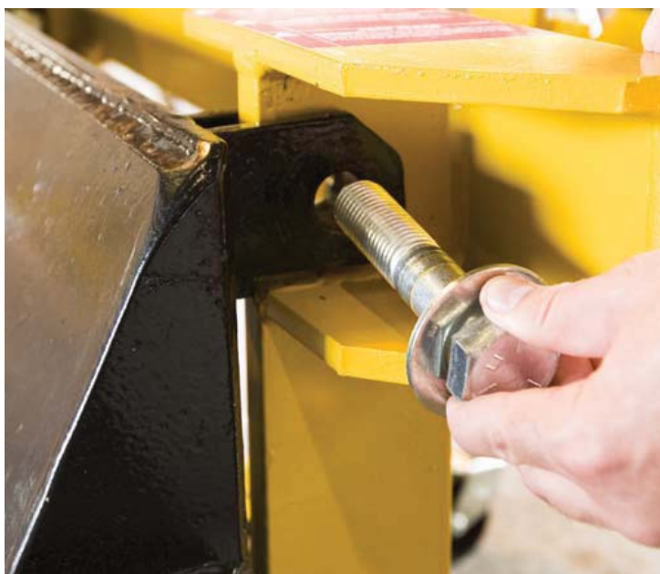
Figure 31.0 MPS 350 Bumper Assembly Bolts Mounting MPS 350 to Truck Frame
