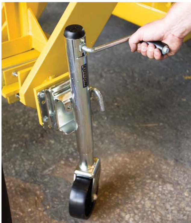
Figure 32.0 Adjusting MPS 350 Height Manually with Jacks
