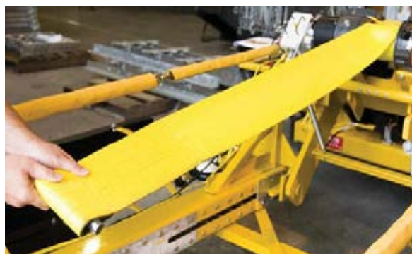
Figure 11.1 Straps Released to Cross Frame
