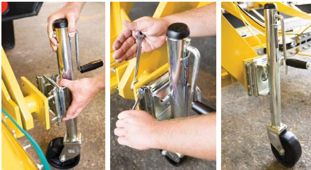
Figure 29.0 Three (3) Jack Attachment Locations - Jacks Attached with Four (4) Bolts/Nuts
