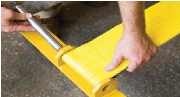
Figure 11.2 Position Strap and Insert 1" (25 mm) Pin
