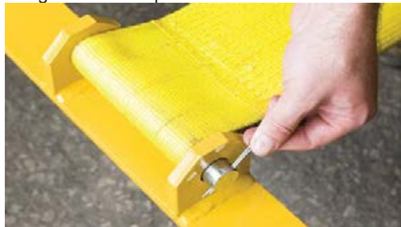
Figure 11.3 Insert Cotter Pin and Secure
