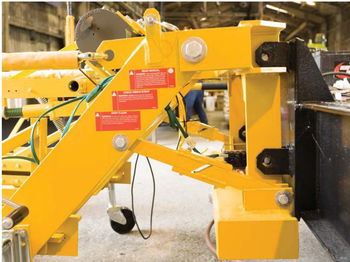
Figure 34.0 Match MPS 350 Bracket Assembly and Bumper Connection Points
