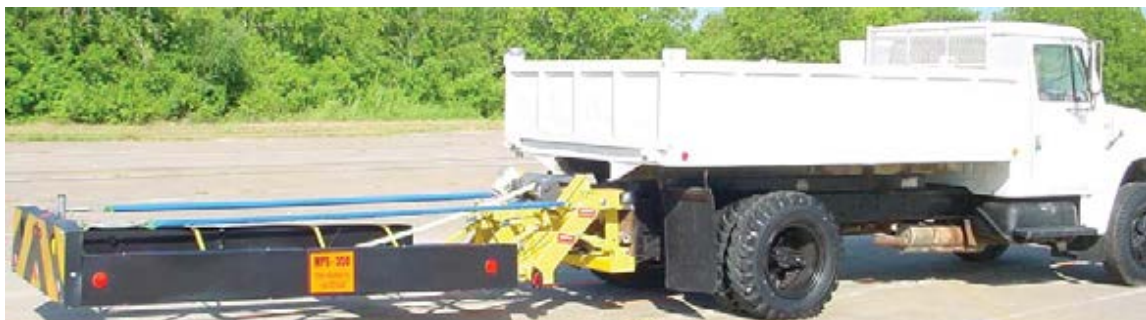
Figure 17.0 MPS 350 in Down (Operating) Position
